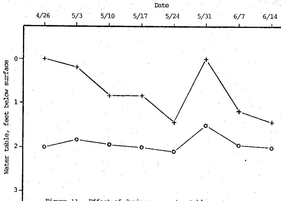
Figure 11. Effect of drainage on water tables, Miner Institute, Spring 1979
