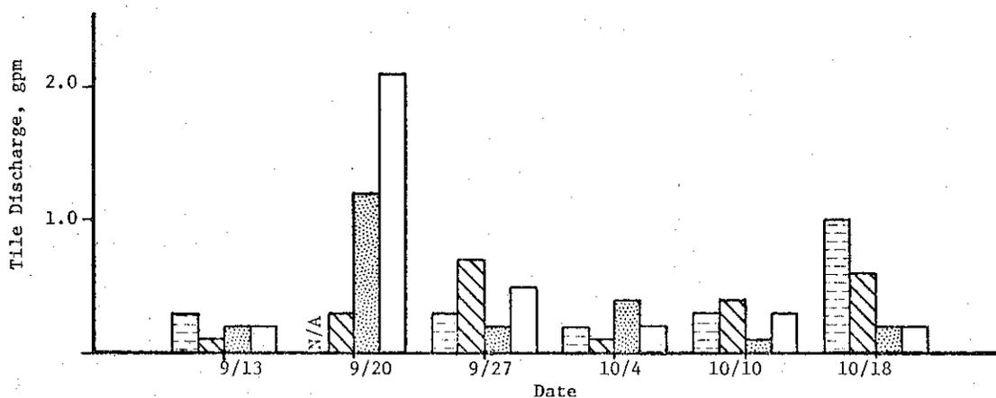
Figure 19. Instantaneous tile discharge rates
