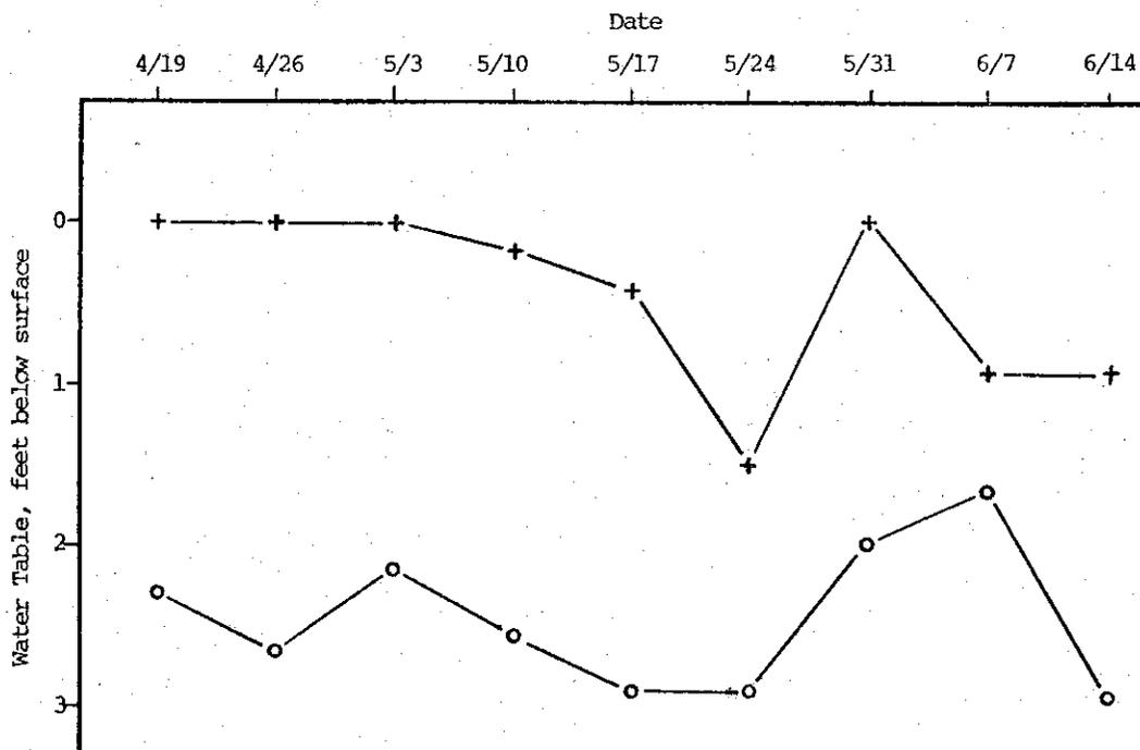
Figure 12. Effect of drainage on water tables Miner Institute, Spring 1979
