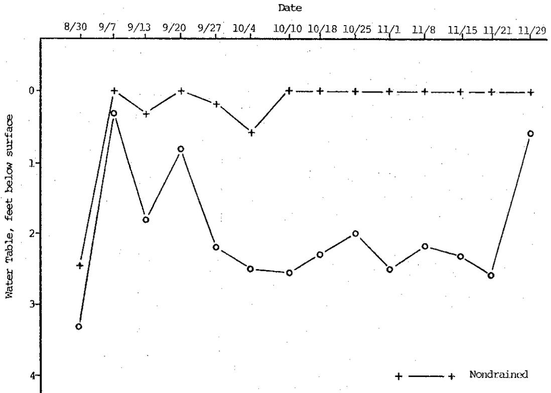
Figure 14. Effect of drainage on water tables
