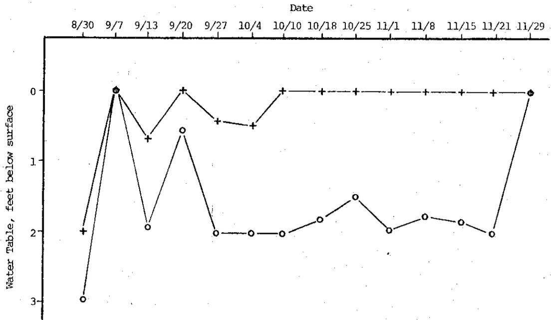
Figure 13. Effect of drainage on water tables.
