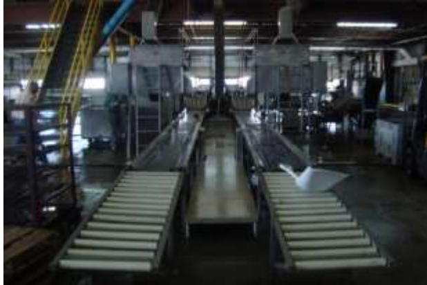
Figure 5 Immersion hydro-cooling ('Dipper'): broccoli boxes are placed on conveyor belts that circulate them in troughs filled with cold water (water and crushed ice)
