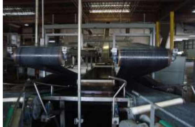
Figure 5 Immersion hydro-cooling ('Dipper'): broccoli boxes are placed on conveyor belts that circulate them in troughs filled with cold water (water and crushed ice)
