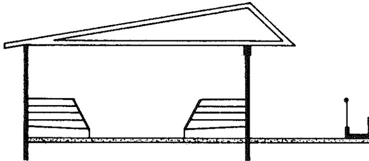
Figure 2. Roof design allows for an open feed area with stalls under cover.
