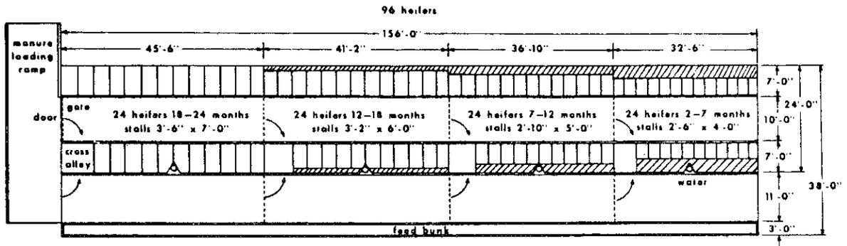
Figure 1. Floor plan shows basic layout for 96-stall heifer barn. Heifers are easily confined in either the stall or feed alley while the other side is being scraped. Note the straight curbs for easy manure handling.
