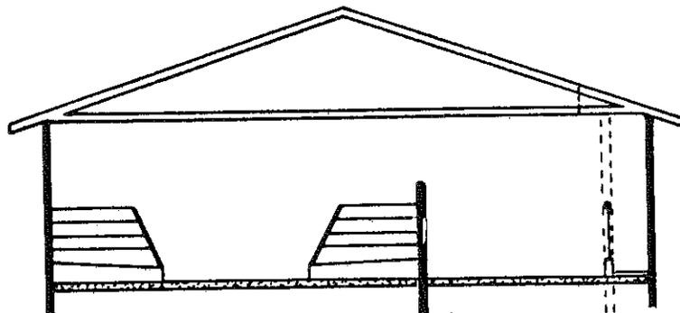
Figure 3. A bunk feeder or wagon can be used in this totally covered system. (Dotted line shows the location of post for wagon feeding).
