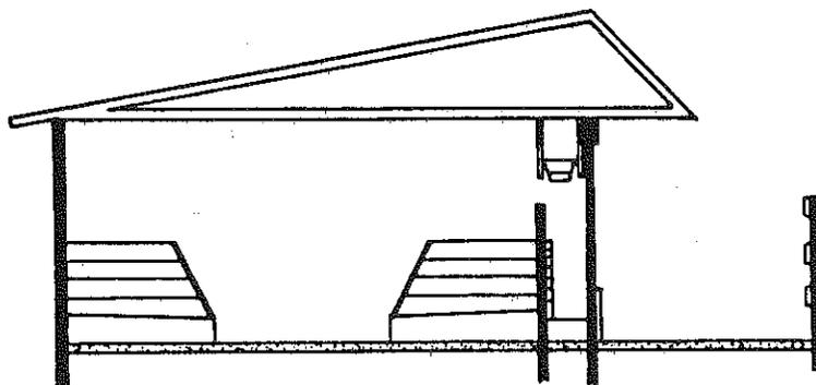
Figure 4. Stalls and bunk are covered while roofed area is kept to a minimum. Heifers eat from open alley.
